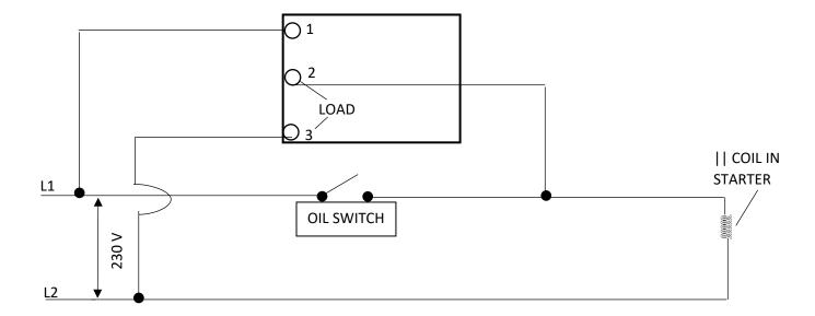
The initial power to your coil is open at the oil switch on start up. This timer allows a 15 second 'by-pass' with power going to #1 and out through #2 on the timer, by-passing the open oil switch. The Oil switch will then close and latch power to the starter coil once the oil pressure is built, before the timer opens #1 to #2 after 15 seconds.
