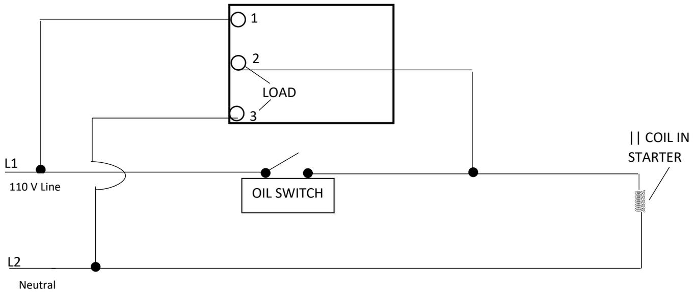
The initial power to your coil is open at the oil switch on start up. This timer allows a 15 second 'by-pass' with power going to #1 and out through #2 on the timer, by-passing the open oil switch. The Oil switch will then close and latch power to the starter coil once the oil pressure is built, before the timer opens #1 to #2 after 15 seconds.
